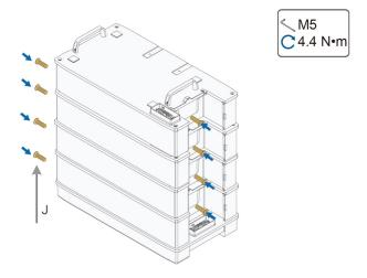
step 7 Connect the switch gear to the base.
