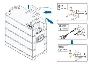
The bracket is mounted on the top battery module.
